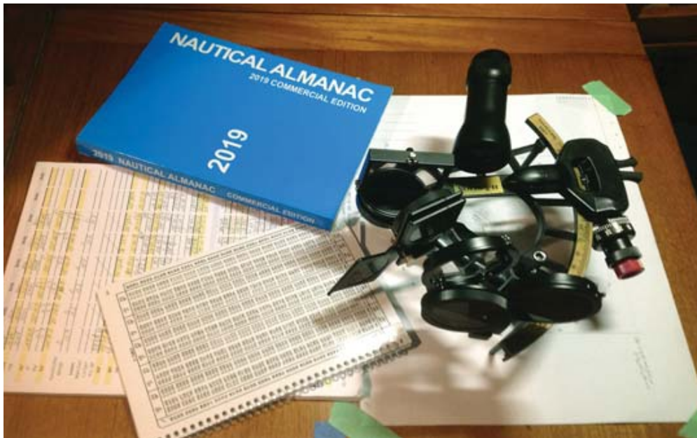
Tools of the trade. I had customised work-forms and laminated, spiral-bound S-Tables (concise sight reduction tables) made up for the trip. I used a superb Cassens & Plath Horizon sextant exclusively throughout the voyage
