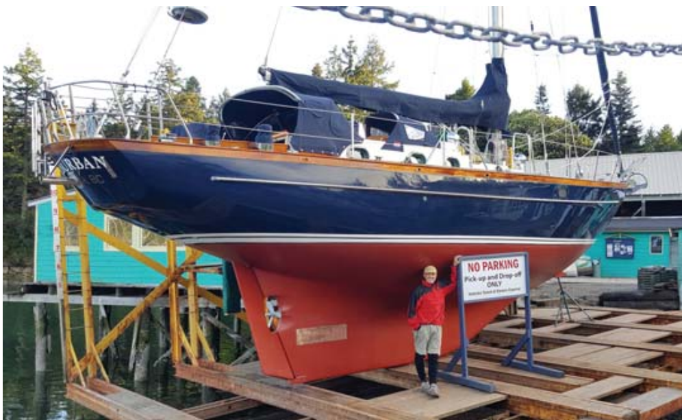
Seaburban on the ways at Silva Bay Shipyard on Gabriola Island, BC, prior to her heading north to Alaska. Her keel and forefoot, narrow beam and long overhangs are testament to her CCA roots
